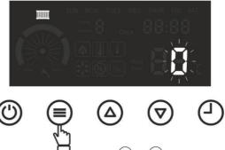
■ For underfloor heating select "0" using  $\bigcirc$  or  $\bigcirc$  keys.
