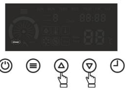
If "shower" and "heating" are selected at the same time, the device operates for DHW and central heating.
