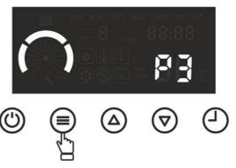
■ Using or keys, the device capacity is set to P1, P2 or P3. Indicator lights change according to the selected capacity.
