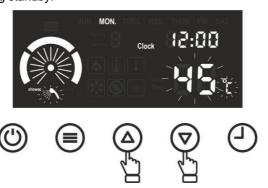
To adjust the DHW temperature during operation for central heating, the operating mode of the device must be changed to DHW heating. At the end of the process, the device should be returned to its previous operating position. (Please see 6.4.8)
