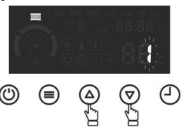
⚠In underfloor heating systems, the "0" setting in this menu cannot be changed since the heating mode is set by qualified personnel from within the device.
