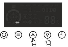
If "shower" is selected, the device only works for DHW heating.
