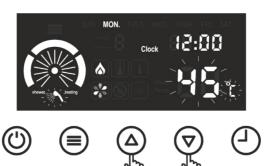
If the operating mode is set to DHW heating, it is also possible to change the boiler temperature during standby.
