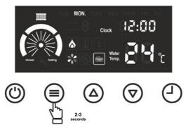
Until "*Timing Time Phase*" appears, press the button at intervals of one second, the time program number starts to flash.
