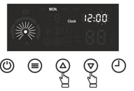
By pressing the button once or by not pressing any buttons for 10 seconds, the settings are saved and the setting menu is exited.
