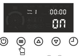
$\blacksquare$  The program start time is determined using  ${\overline{\heartsuit}}$  or  ${\overline{\triangle}}$  keys.
