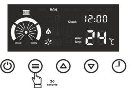
Press the button at intervals of one second until the "Timing Time Phase" appears, the time program number starts to flash..
