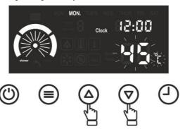
In order to adjust the domestic water temperature during operation for central heating, the operating mode of the device must be changed to domestic water heating. At the end of the process, the device should be returned to its previous operating position (please see 6.4.8). 2 seconds after the adjustment is completed, the instantaneous operating temperature and the "*Water Temp*" text are displayed on the screen.
