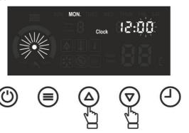
By pressing the button once or by not pressing any buttons for 10 seconds, the settings are saved and the setting menu is exited.
