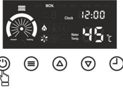
⚠ In underfloor heating systems, the temperature should never be set above 55°C.
