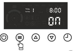
$\blacksquare$  The programme start minute value can be determined using  $^{\bigcirc}$  or  $^{\triangle}$  keys.
