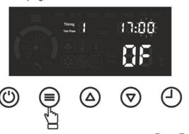
$\blacksquare$  The programme end minute value is determined using  ${\overline{\bigtriangledown}}$  or  ${\overline{\bigtriangleup}}$  keys.
