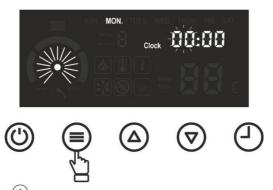
■ Press the  $\bigcirc$  or  $\bigcirc$  buttons at one second intervals to set the time between 0 and 23.
