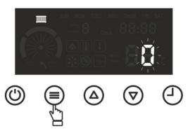
■ For underfloor heating select "0" using the or the keys.
