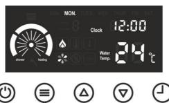
■ The key is pressed at intervals of one second until the appears, the heating mode option indicator starts to flash.
